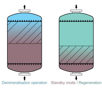
**Regeneration** The exchanger material must be regenerated when fully exhausted.
