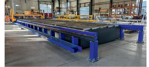
Operated at a relatively high air extraction rate of up to 9,600 m<sup>3</sup>/h, the sequential extraction system in the cutting table prevents air pollution on shop floors, thus ensuring a high work safety standard. The rapid air extraction rate requires a suitably large intake air volume. The heat from the extract air is therefore used directly in the extraction system to preheat the intake air, thus optimising energy usage. **This extraction system has a thermal efficiency of almost 100%.**
