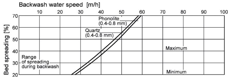
The filter rinsing must be done so that the filter material is in a state of suspension. Only in this way can the held-back substances also be reliably
