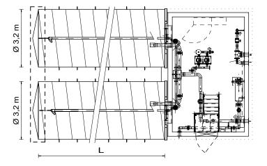
Basic layout: Pipe tank with two tanks and concrete control compartment.
