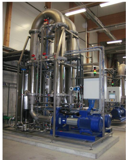
Ultrafiltration with ceramic Multibore tubular membranes
