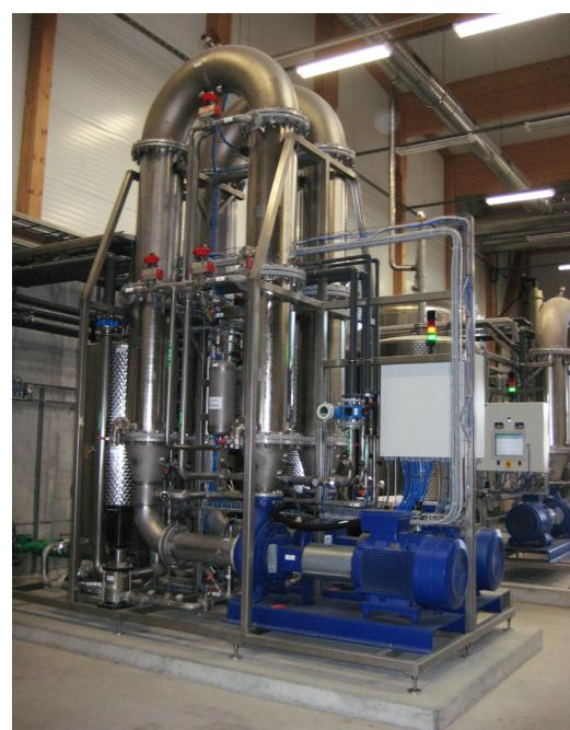
Ultrafiltration with ceramic Multibore tubular membranes
